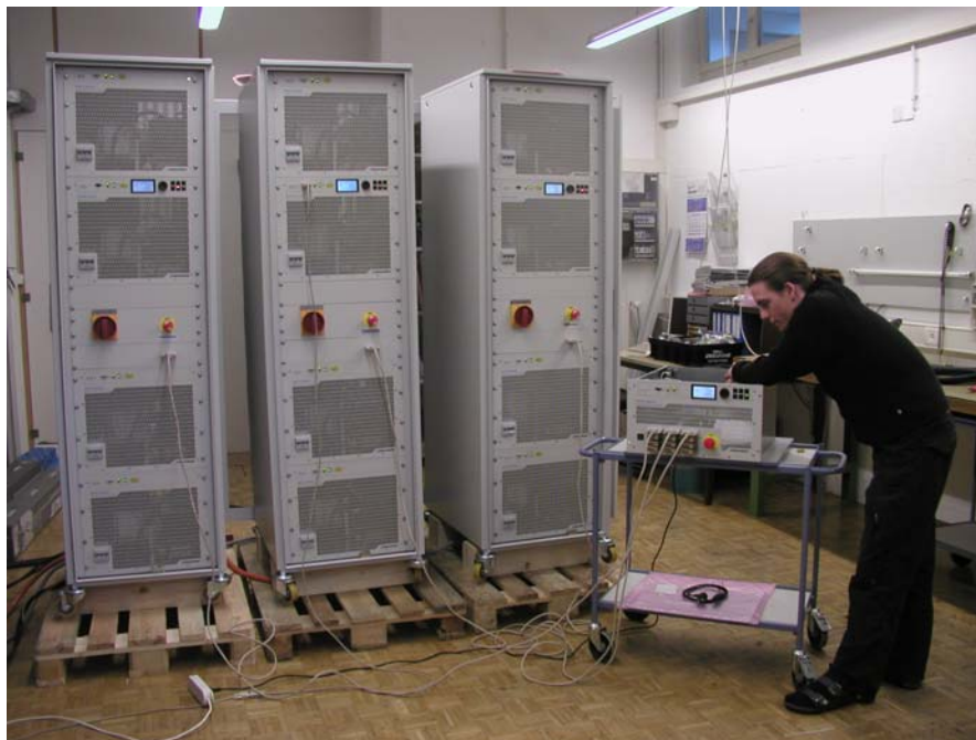
Picture 7: Final adjustments on a 3 x 128 kW system
