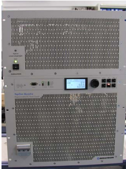
Picture 4: TopCon (below) and TC_LIN units form a 1000V/32 kW stack
